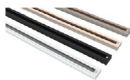
K5-3 Single Circuit/Two Circuit Track Single Circuit Track is rated for 2400W Features 12-gauge copper conductors and a separate ground conductor. Two circuit track includes 12-gauge copper conductors and features a double load capacity at 4800W max. Single/Two Circuit Track is available in white, black and satin nickel finishes, and in 4, 6, and 8-foot sizes, and can also be field cut to your preference.
